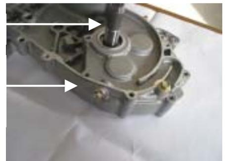
b) Remove the oil seal, and drive out the bearing.
