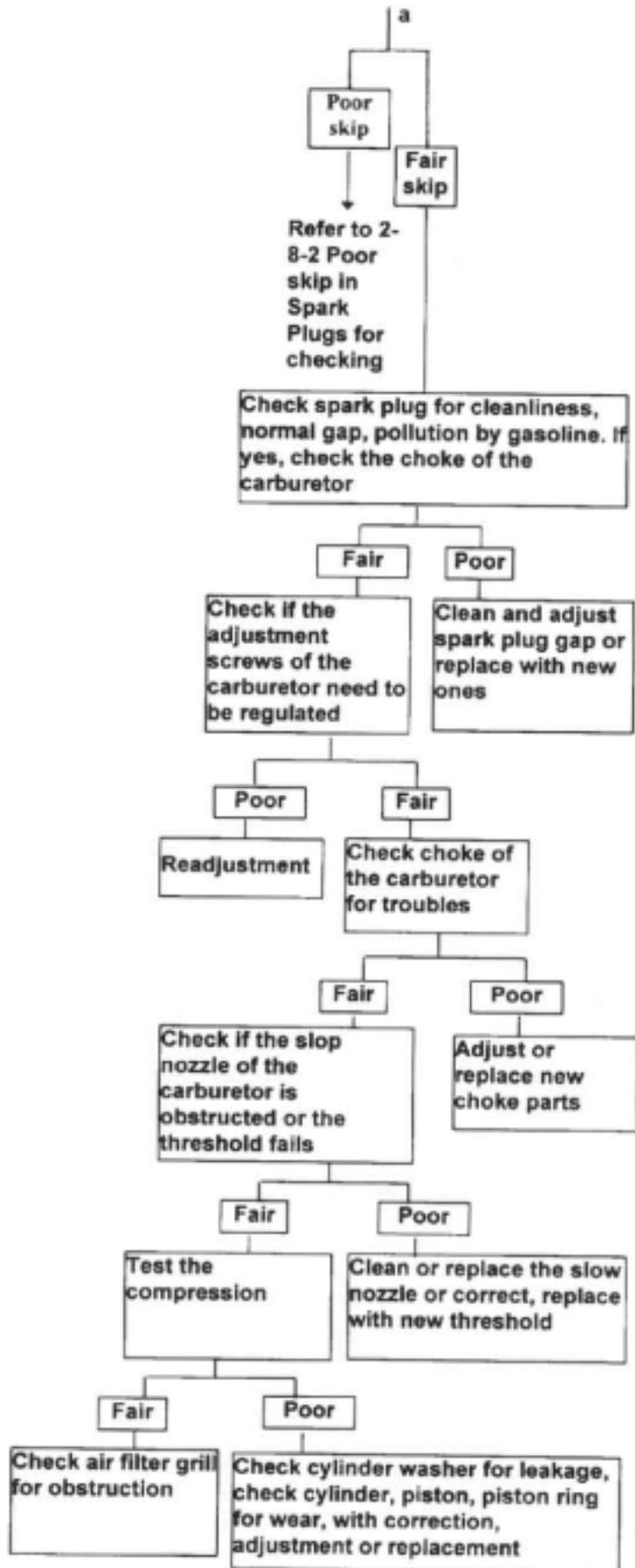
● **Troubleshooting for Failure in Starting Carburetor**
