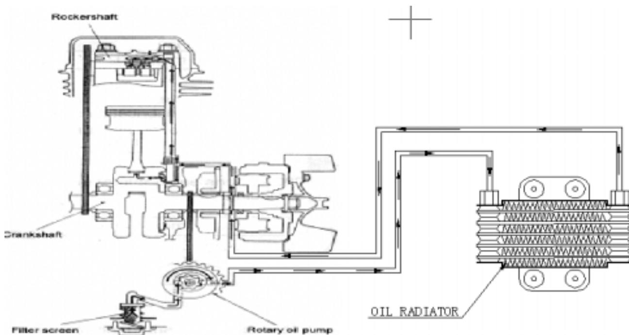
After the lubrication oil crosses the filter screen, it is pumped by the rotator oil pump; some of the oil goes into the big end of the connecting rod, and splashes on the cylinder wall and the small end of the connecting rod; all the other goes through the oil passages, such as the shaft neck of the camshaft, and splashes on the cam rockshaft and cam chain. The lubrication oil that falls back into the oil groove can be re-circulated.
