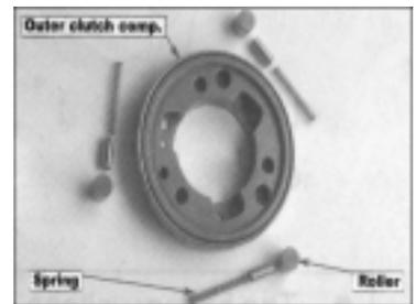
d) Apply some oil on the needle bearing and drive gear, and then put the outer clutch component on.
