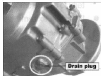
**Recommendation:** before draining the final gear oil, please warm the engine for at least 10 minutes.
