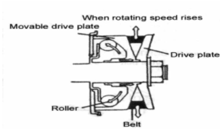
The picture shows the structure of the driven belt pulley. The clutch showed in the picture is the automatic dry centrifugal weight clutch.
