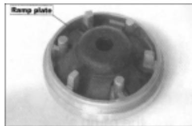
c) Put the drive plate hub into the drive plate.
