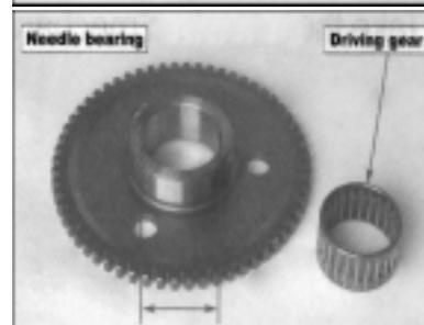
b) Inspect the condition of the needle bearing. It should be replaced if there is any damage.
