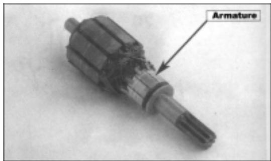
● Please don't use the sandpaper to grind the armature, or wash it in any solvent that can dissolve or damage its insulation.
