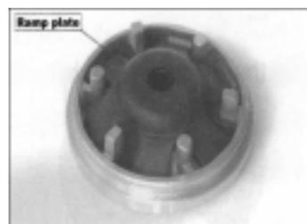
e) Remove the centrifugal rollers.
