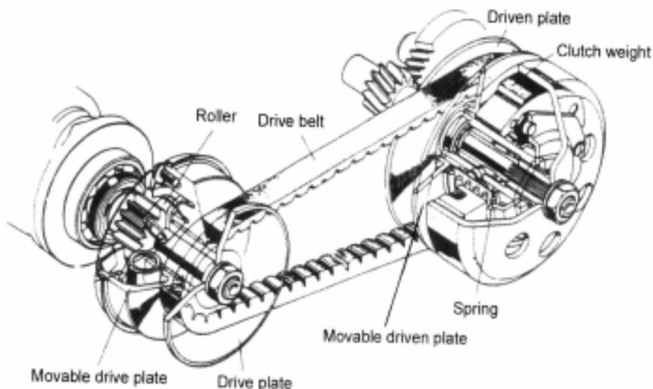
Its basic operational principle is to realize the automatic CVT by the diameter changes (the transmission ratio changes) of the driving and driven belt pulley.
