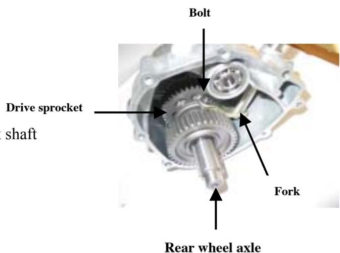
d) Remove the center shaft comp. and idle gear comp.;
