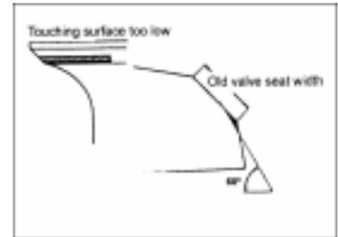
c) Finally, grind the working face of the valve seat to the specific width with a 45° grinding cutter.
