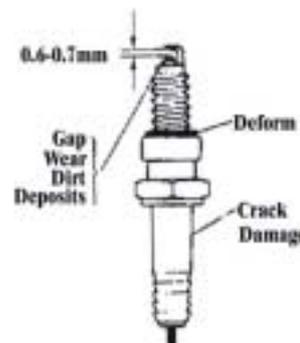
**Note:** The electrodes should be kept clean and free of carbon. The presence of carbon or excess oil will greatly deter the proper engine performance.
