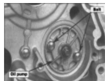
f) Remove the screws, and disassemble the oil pump.
