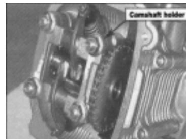
f) Remove the camshaft holder and dowel pin;
