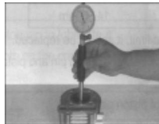
The least measured dimension is the cylinder bore, the data measured at the most upper position is the largest diameter, and the data measured at the lower position is the smallest diameter. At the same cross section, measure the difference of diameter between the two points mutually perpendicular, which is the circularity of the cylinder.
