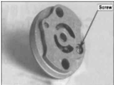
c) Tighten the oil pump plate screws;
