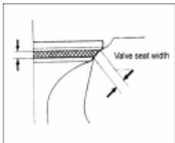
When the abrasion causes the valve seat width uneven, too wide or too narrow, it will result in bad contact between the valve and valve seat, and can't seal tightly. At this time, it must be reamed with a customized valve seat-grinding cutter.
