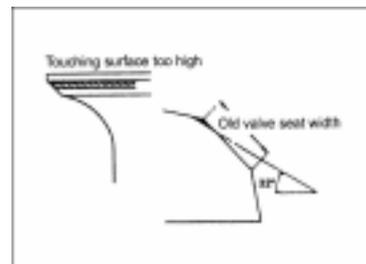
b) If the contact position is too high, then cut out some of the upper part of the valve seat with a 32° grinding cutter to reduce the working face of the valve seat; if the contact position is too low, then cut out some of the lower part of the valve seat with a 60° grinding cutter to raise the working face of the valve seat.
