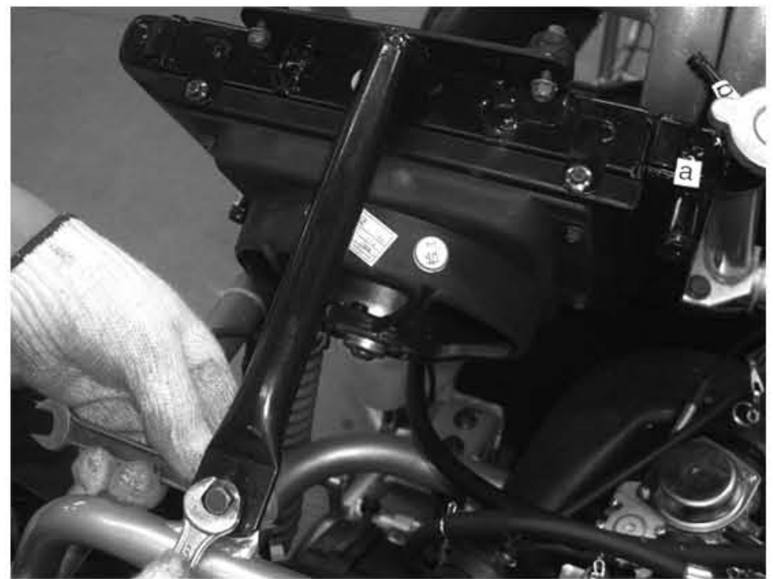
16.Install water tank
