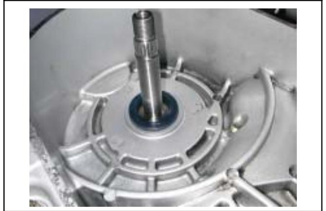
Apply by oil seal driver (27×42×7), oil seal will knock into location.
