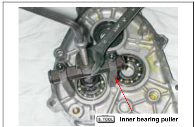
Remove cir clip of final shaft out side bearing.
