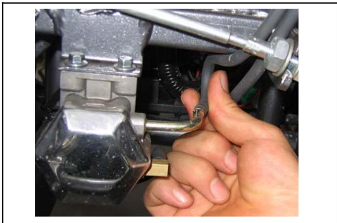
Remove vacuum tube from the fuel pump.
