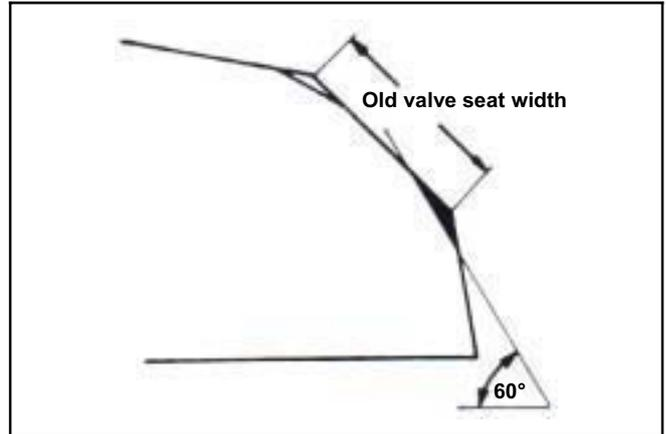
Use 45° cutter to grind the valve seat to specified width.
