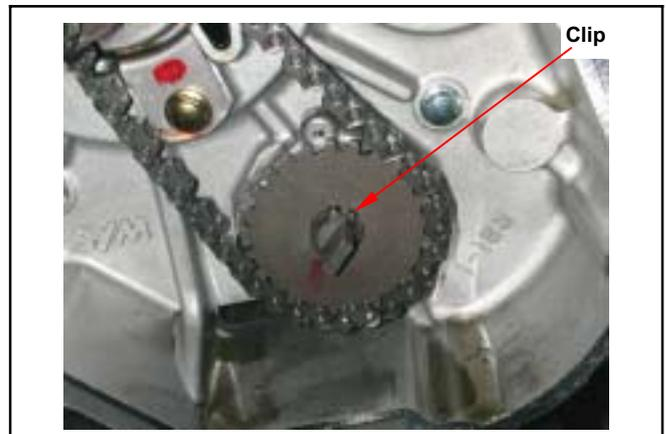
Install starting gear and generator.
