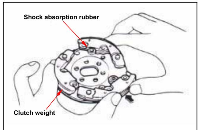
Install the spring into groove with pliers.
