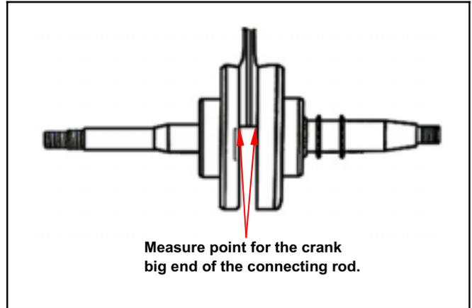
Measure the clearance of the large end in the vertical direction.
