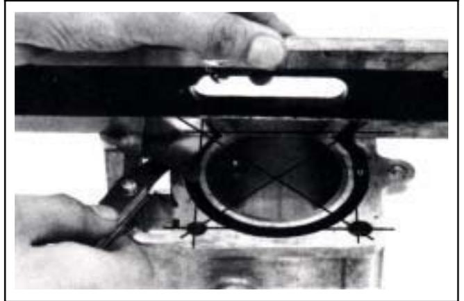
Measure clearance between piston rings and grooves.
