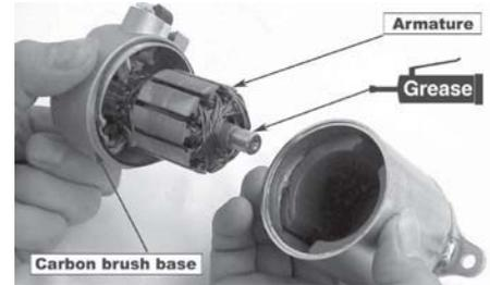
Do not damage the contact area of the carbon brush and the armature. When installing, do not damage the lip of the dust seal.
