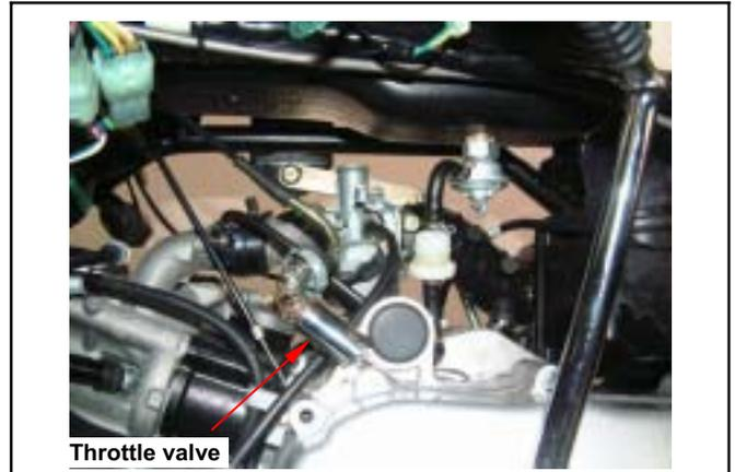
Disconnect the throttle cable from the throttle valve and remove the valve spring. Remove the fuel needle clamp and fuel needle.
