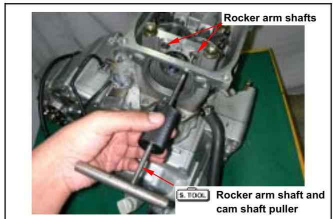
Remove cam shafts.
