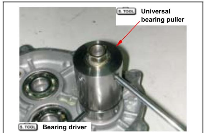
Install new oil seal and bearing driver into gear box covers inner side.
