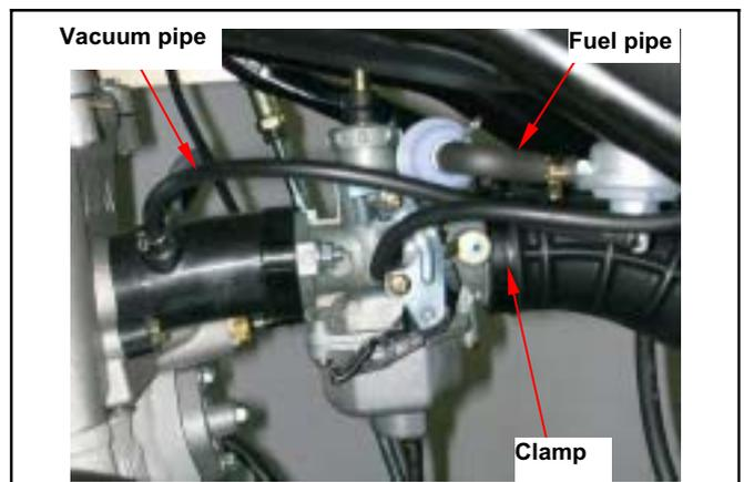
Remove the carburetor upper parts from the carburetor.
