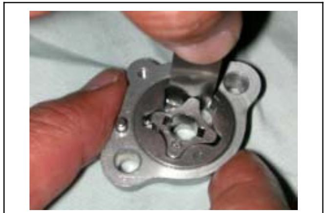
Check clearance between rotor side face and pump body
