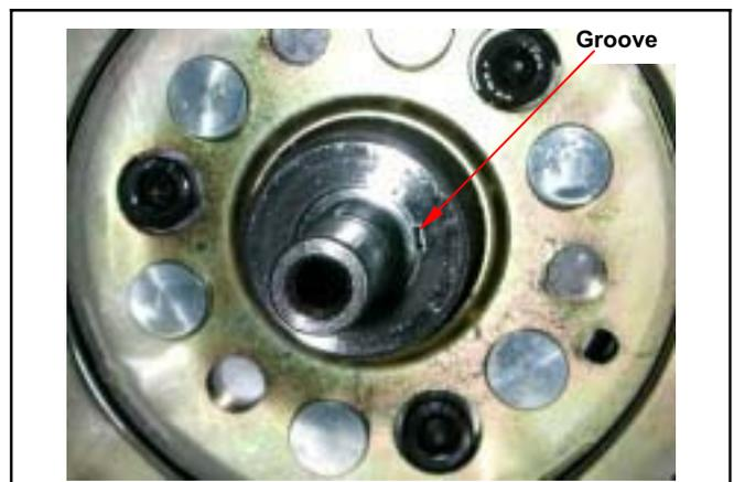
Hold the flywheel by drive face with universal holder, and tighten flywheel nut.
