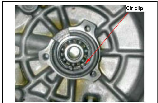
Remove the cir clip, and then remove bearing.
