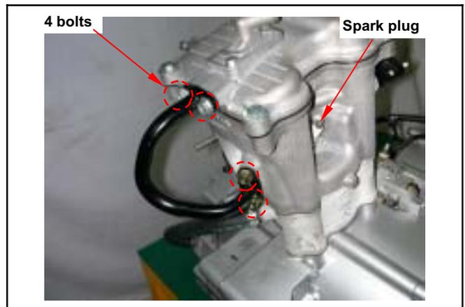
Remove the side cover mounting bolts of cylinder head, and then take out the side cover.
