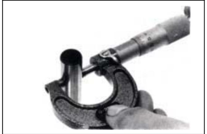
Measure the inner diameter of connecting rod small end.
