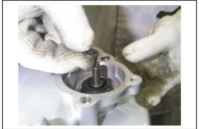
Install the impeller onto the water pump shaft and tighten.
