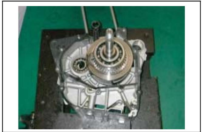
Remove gasket and dowel pins.
