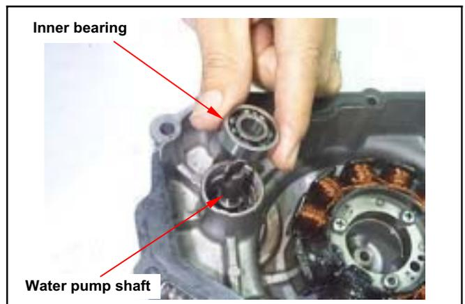
Install the cir clip to hold the inner bearing.
