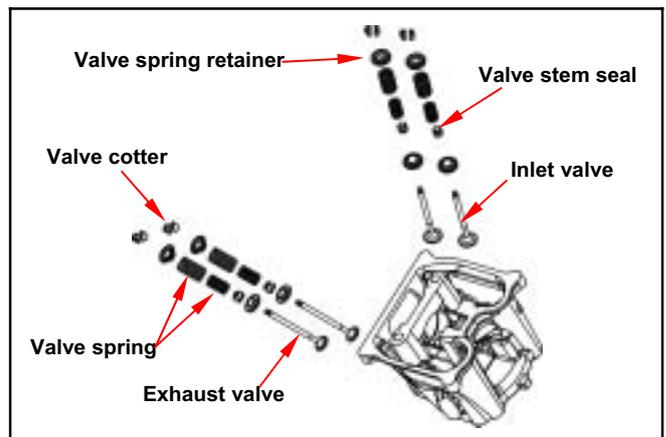
Use a valve cotter removal & assembly tool to press the valve spring, and then remove valves.
