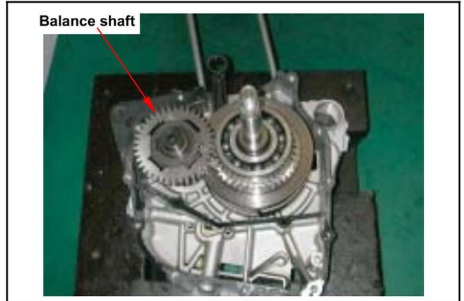
Remove crankshaft from right crankcase.
