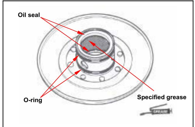
Install the movable driven face onto driven face.
