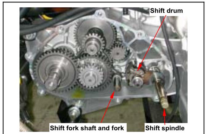
Remove final shaft, counter shaft, and reverse shaft.
