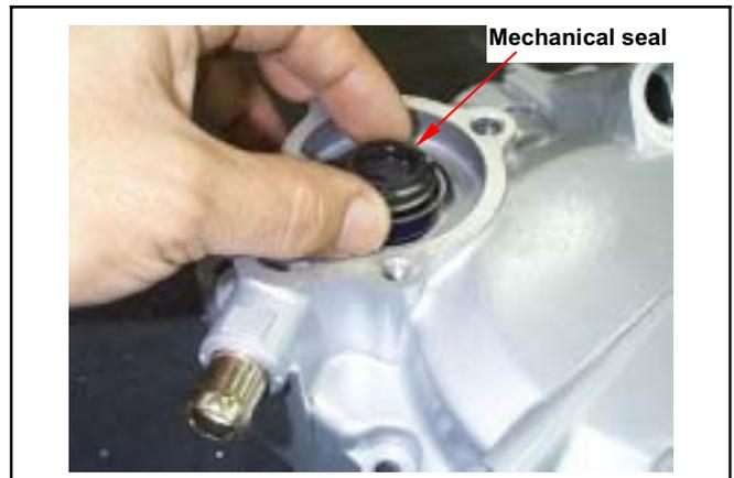
Install the mechanical seal onto the right crankcase.
