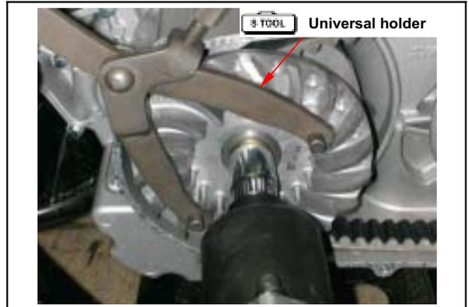
Hold clutch outer with universal holder, and remove nut, bearing stay collar and clutch outer.
