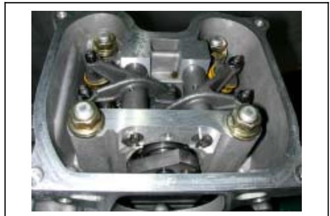
Install rocker arm pin mounting plate.
