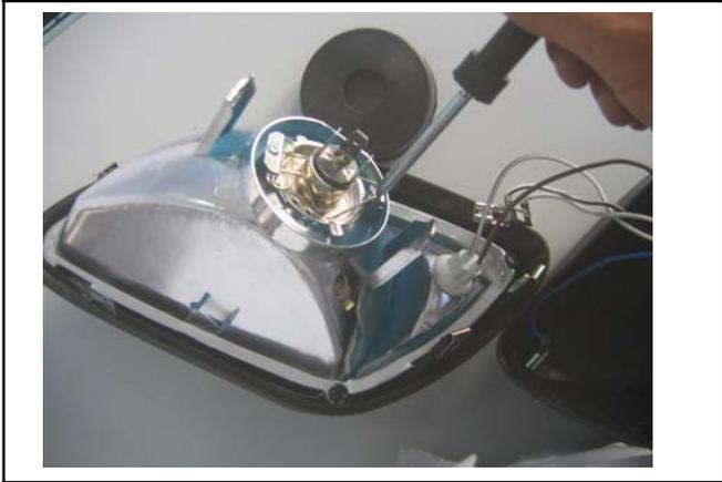
Install dust boot and wiring connectors.
