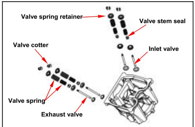
Use a valve cotter removal & assembly tool to press the valve spring, and then remove valves.
