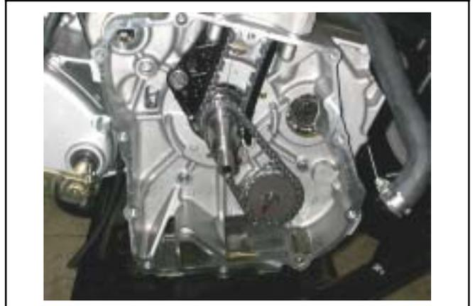
Remove cir clip and take out oil pump driving chain and sprocket.
