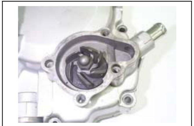
Install the dowel pin and new gasket. Install the water pump cover with 4 bolts.
