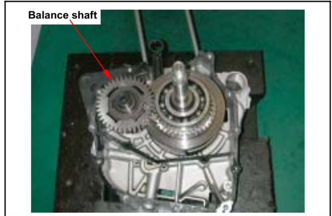
Remove crankshaft from right crankcase.
