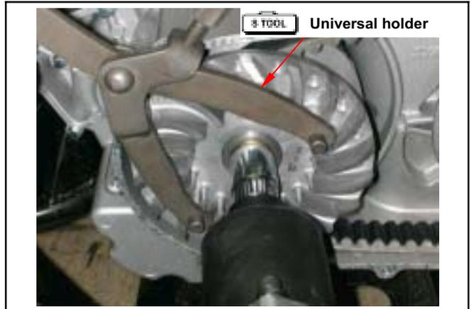
Remove movable drive face comp and drive face boss from crankshaft.
