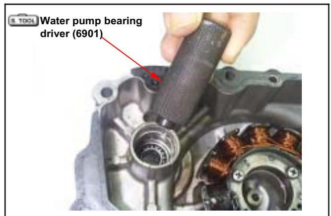
Mount the water pump shaft and the inner bearing to the right crankcase cover.
