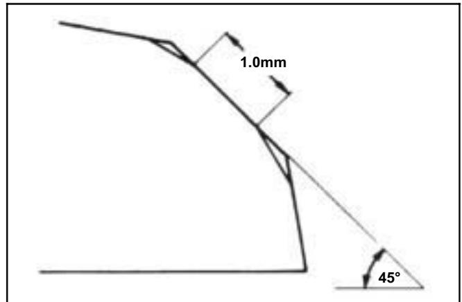
Coat the valve seat surface with red paint.
