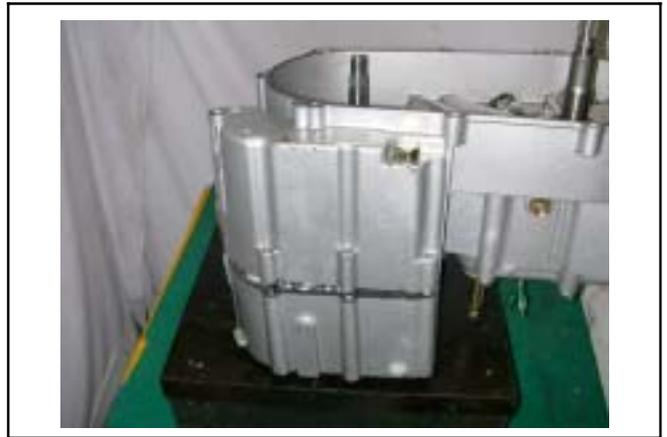
Tighten 11 bolts on the left crankcase.
