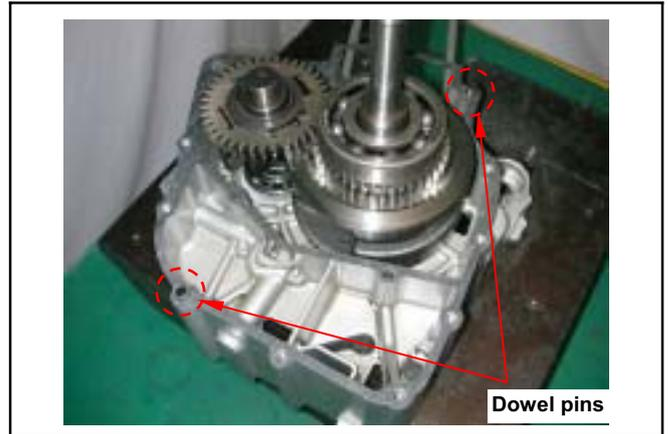
Install the left crankcase onto the right crankcase.
