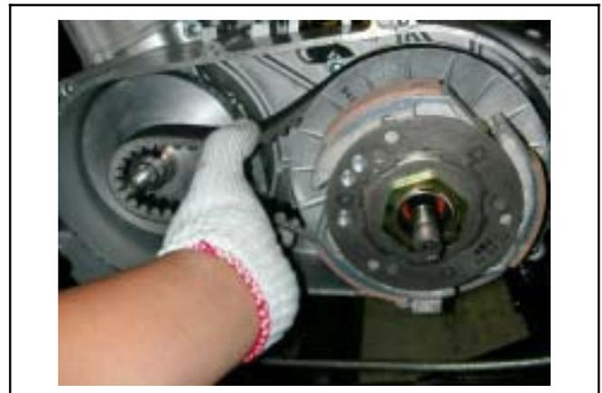
Install the clutch outer and bearing stay collar.
