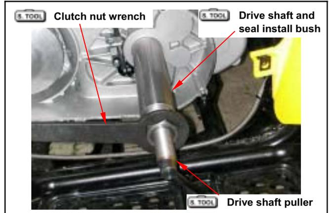
Apply with grease onto new drive shaft oil seal lip, and then install the oil seal.
