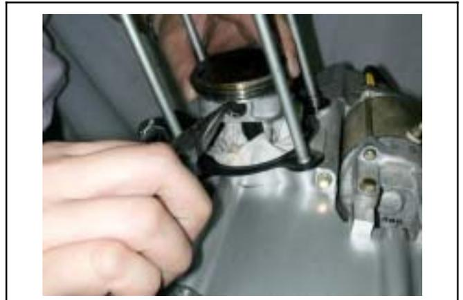
Remove cylinder gasket and dowel pin.
