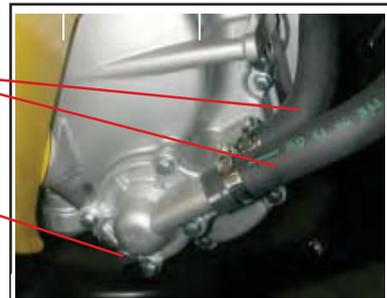
Remove coolant inlet hoses from water pump.
