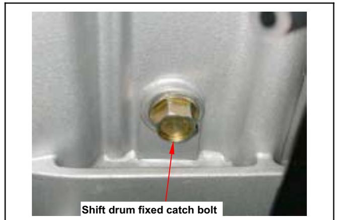
Remove shift spindle, shift fork shaft, shift fork, and shift drum.
