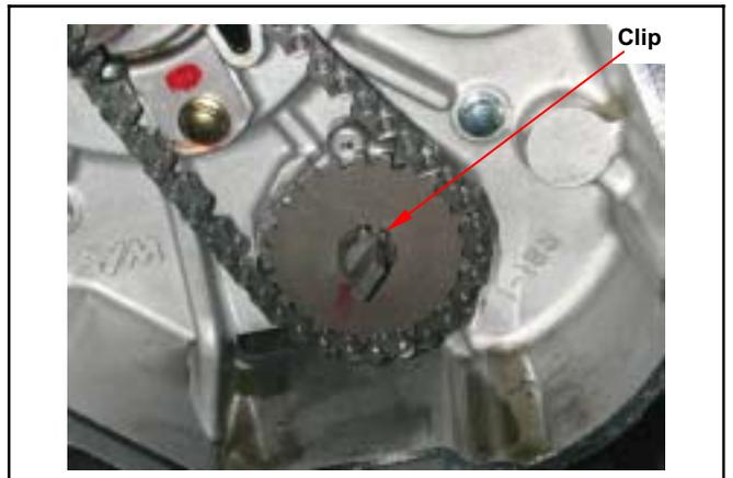
Make sure that pump shaft can be rotated freely. Remove 2 screws on the oil pump, and then remove oil pump.
