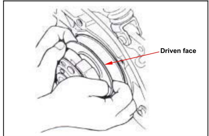
Install the driven pulley with belt onto drive shaft.
