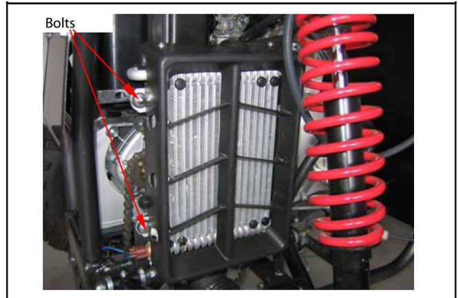
Remove coolant outlet pipe.
