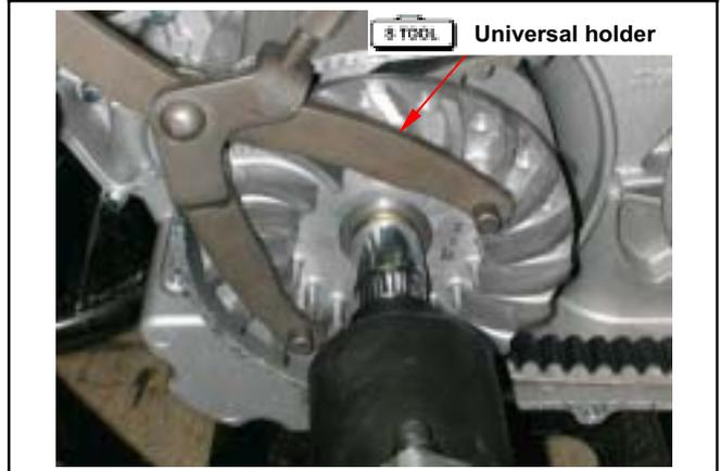
Remove movable drive face comp and drive face boss from crankshaft.
