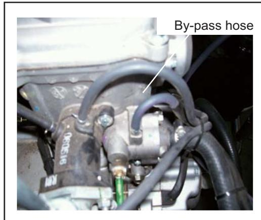
2. With the engine running at idle fill the radiator with coolant. Fill the radiator until coolant comes out of the by-pass valve. When **ONLY** coolant comes out of the by-pass valve and there are no air bubbles in the coolant, reconnect the by-pass hose.
