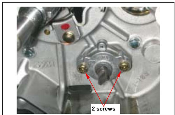
Install oil pump drive chain and sprocket, and then install cir clip onto oil pump shaft.
