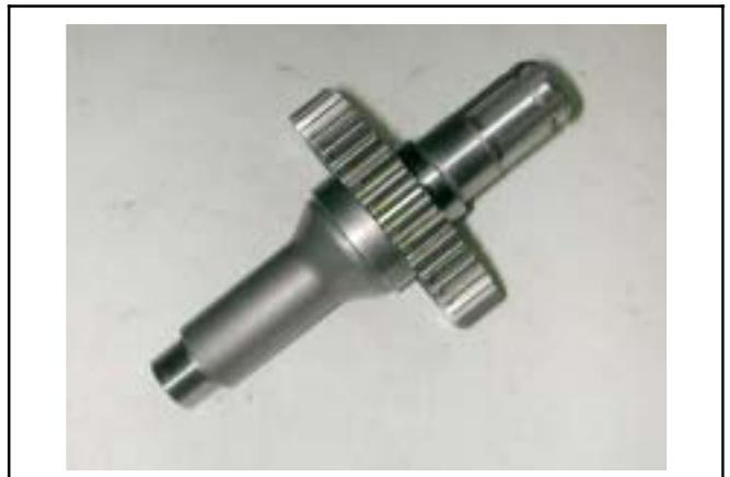
Check bearings on gear box and gear box cover. Rotate each bearing's inner ring with fingers. Check to see if bearings turn smooth and silent. Check to see if bearing outer ring is mounted on gear tightly. If bearing rotation is uneven, noisy, or has loose bearing mount, then replace it. Check oil seal for wear or damage, and replace it if necessary.
