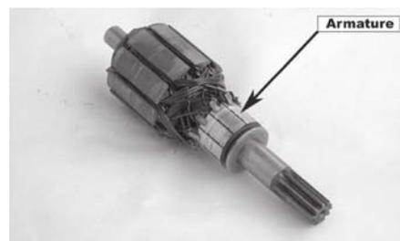
Do not use sandpaper to grind the armature surface, nor wash it in any solvent which can dissolve or damage its insulation.
