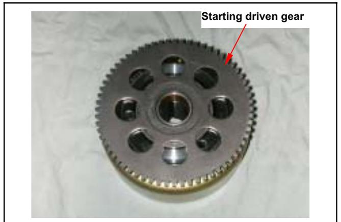
Remove 3 socket bolts, and then remove one way clutch.
