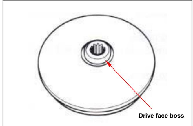
Install movable drive face comp. onto crankshaft.
