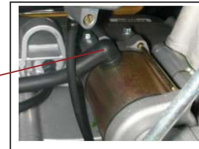
Remove the spark plug wire.
