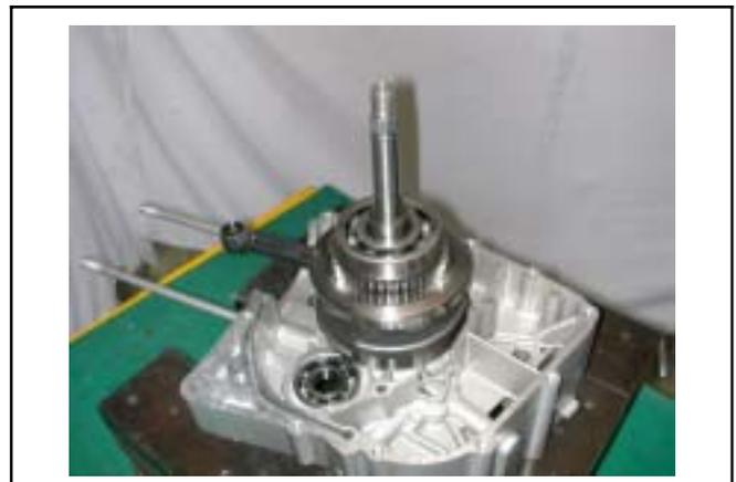
Align the position mark on the balance shaft drive gear with that of balance shaft driven gear, and then install balance shaft onto right crankcase.
