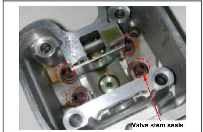
Clean carbon deposits in combustion chamber.
