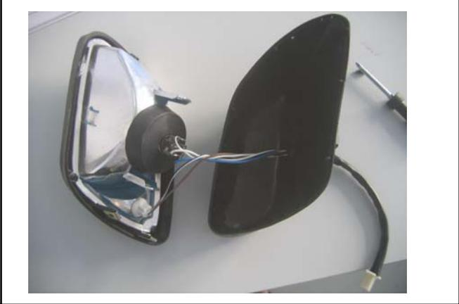
Remove wiring connectors.
