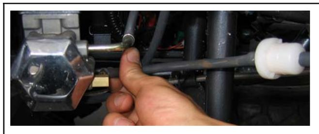
Put out the pump's exit tube.
