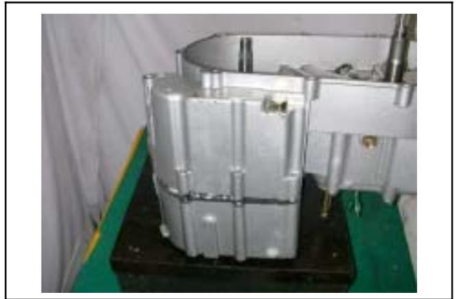
Tighten 11 bolts on the left crankcase.
