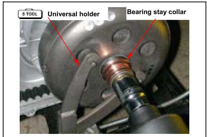
Push the drive belt into belt groove as diagram shows so that the belt can be loosened, and then remove the driven pulley.
