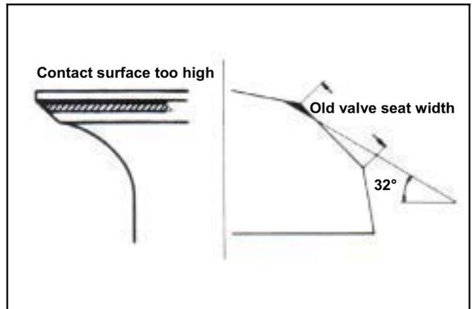
If the contact surface is too high, grind the valve seat with 32° cutter.
