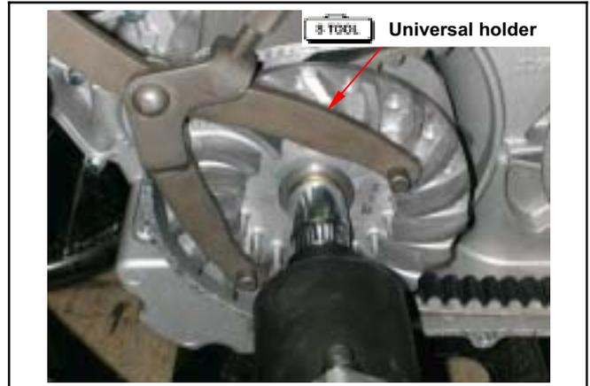
Hold clutch outer with universal holder, and remove nut, bearing stay collar and clutch outer.
