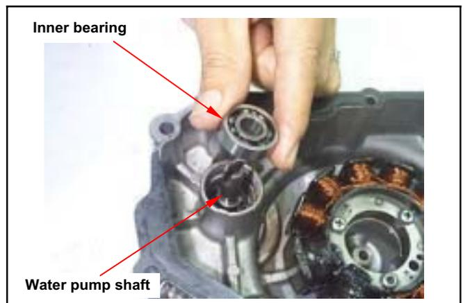
Install the cir clip to hold the inner bearing.
