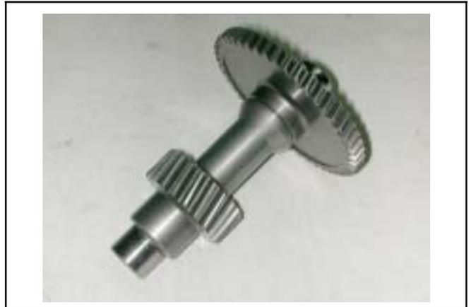
Check to see if the final shaft and gear are burnt, worn, or damaged.
