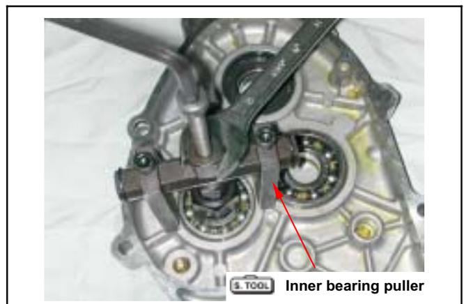
Remove cir clip of final shaft out side bearing.
