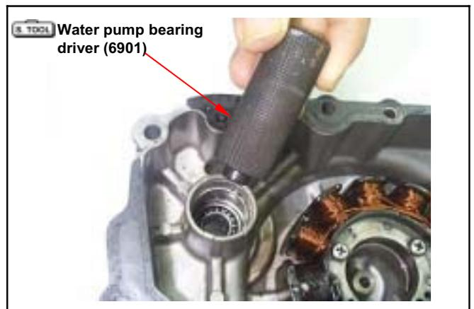
Mount the water pump shaft and the inner bearing to the right crankcase cover.
