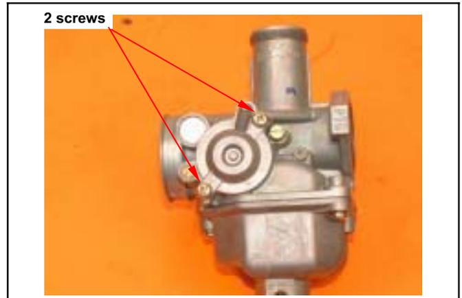
Remove air cut-off valve cover, spring and valve.
