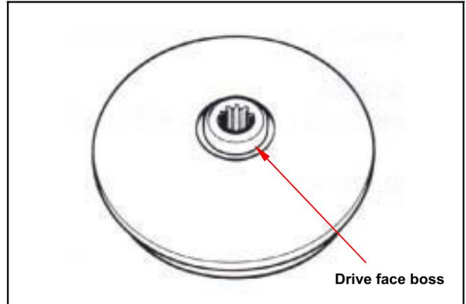
Install movable drive face comp. onto crankshaft.
