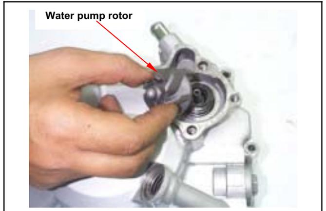
Install the dowel pin and right cover gasket. The rotation water pump impeller, causes the water pump drive shaft scoop channel, aligns the oil pump drive shaft flange, install the right crank case. (9 bolts)
