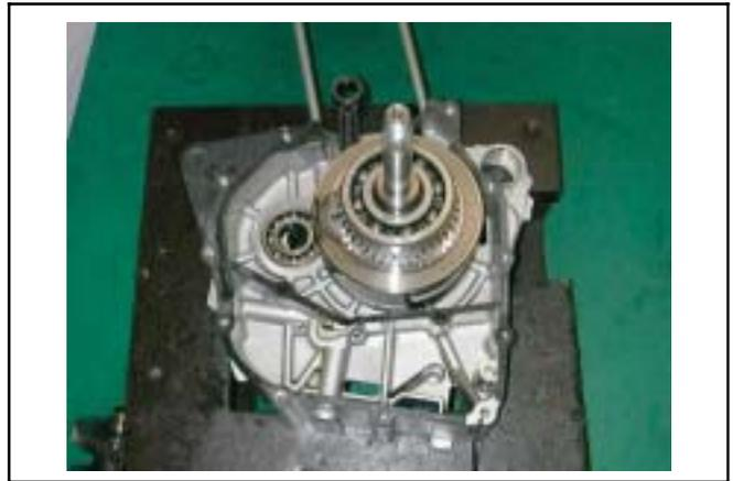
Remove gasket and dowel pins.
