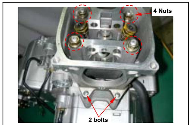
Install camshaft into cylinder head, and install rocker arm and rocker arm shaft.
