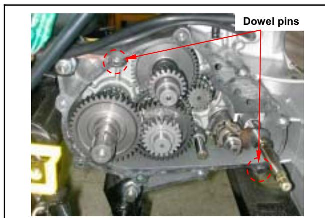
Install gear box cover and bolts, and tighten.
