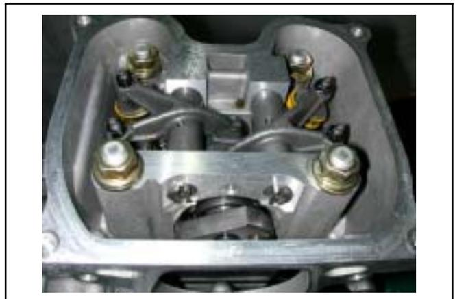
Install rocker arm pin mounting plate.
