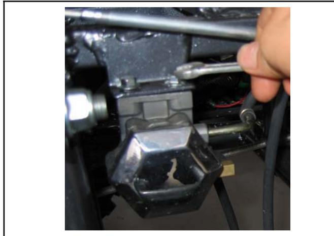
Turn off fuel petcock, then pull out the fuel intake line.
