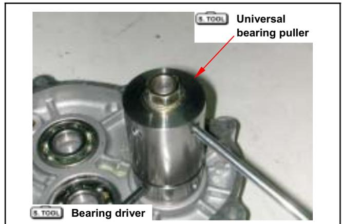
Install new oil seal and bearing driver into gear box covers inner side.
