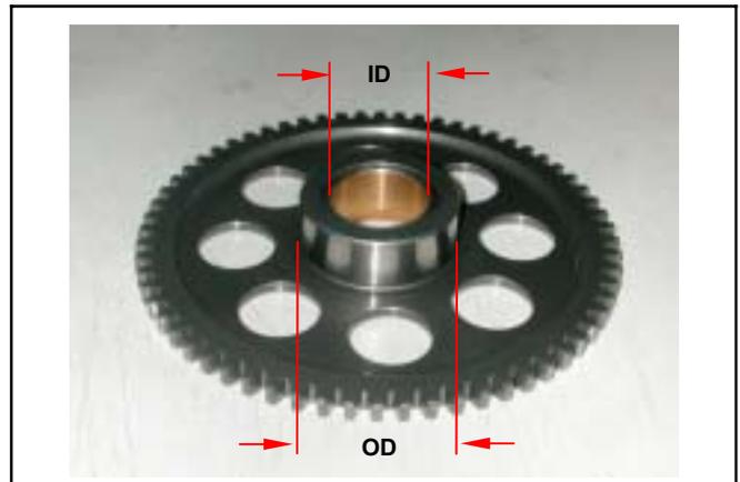
Check the starting reduction gear and shaft for wear or damage.
