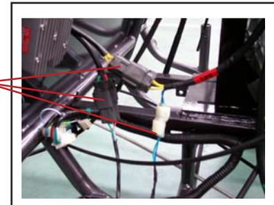
Remove starter motor wire.
