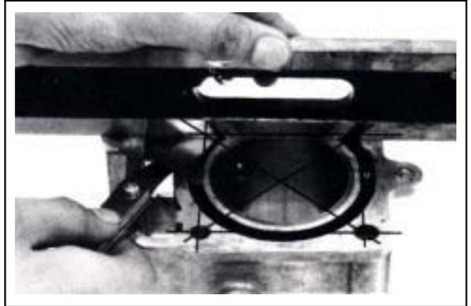
Measure clearance between piston rings and grooves.
