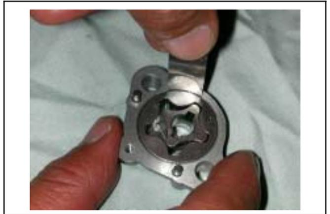
Check clearance between inner and outer rotors.
