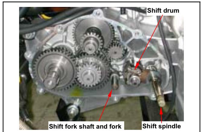
Install shift drum fixed catch ball, spring and bolt, onto gear box.
