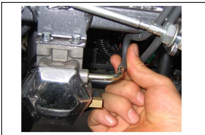
Remove vacuum tube from the fuel pump.
