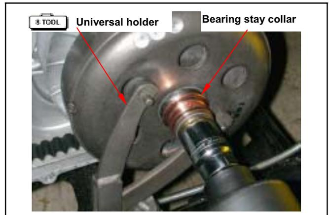
Install the drive face, washer and drive face nut.
