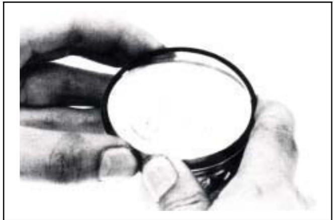
Place piston rings into cylinder below 20 mm of cylinder top, respectively. In order to keep the piston rings in horizontal level in cylinder, push the rings with piston.
