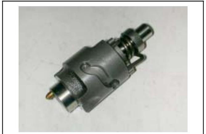
Check if the shift fork and shaft is worn or damaged.
