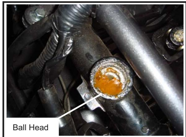
d. Fill steering gear box with grease after cleaning the dust. Replace the ball joint if it is loose or not smooth.
