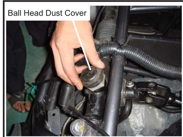
c. Check steering cover on sides of steering gear box and grease the ball head.
