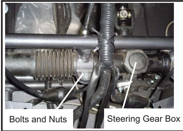
b. Remove and check ball head dust cover and steering gear box for wear.
