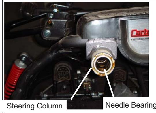
b. Loosen steering shaft, clamp nut and steering gear box.
