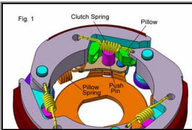
The strength of grip force of HiT clutch [Fig.1, perspective view] is determined not only by the centrifugal force and the friction coefficient of clutch weight, but most importantly by the compression mechanism—push pin & pillow system—of the HiT. The push pin can receive the torque from the engine and then compresses the clutch weight to grab the clutch bell very tightly. Thus, the grip force
