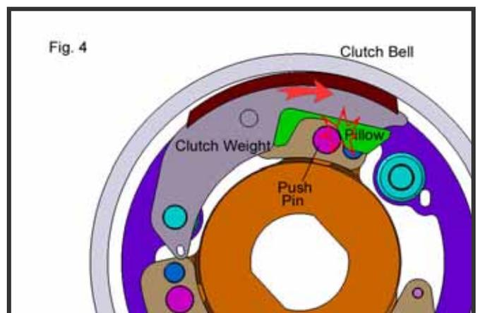
When the friction resistance is higher than the predetermined distortion strength of pillow spring, the pillow spring will be deformed or extended, and the Push Pin will thrust into the Pillow [Fig.4, the push pin is actuated and pressed against the pillow] to compress the clutch weight to grab the clutch bell/outer very tightly.
