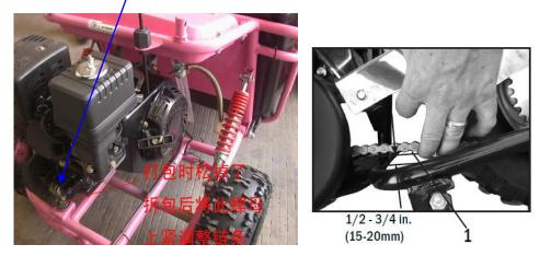
B. If after step. 1 tightening the nut of chain adjustor the chain is still too loose or too tight, <u>another nut at the underpart</u> <u>of chain adjustor</u> must be adjusted accordingly.
