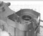
j) Remove the oil seal from the left crankcase.
