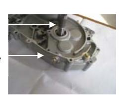
b) Remove the oil seal, and drive out the bearing.
