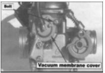
The bottom side of the vacuum membrane should be aligned with the carburetor, and the topside should be aligned with the vacuum membrane.
