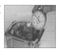
• When the abrasion of the valve guide exceeds the use limit, it should be replaced; after replacing a new valve guide, the valve retainer must be adjusted.
