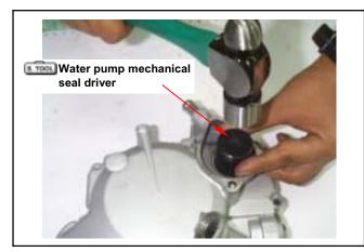
Install the new inner seal onto the right crankcase. **Special tools:**
