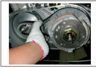
Install the clutch outer and bearing stay collar. Hold the clutch outer with universal holder, and then tighten nut to specified torque value.
