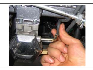
Remove vacuum tube from the fuel pump.
