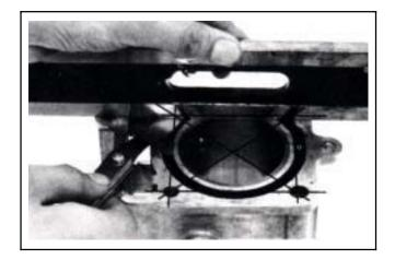
Measure clearance between piston rings and grooves.
