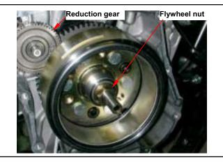
Remove left crankcase cover. Hold the flywheel by drive face with universal holder.
