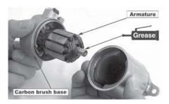
Do not damage the contact area of the carbon brush and the armature. When installing, do not damage the lip of the dust seal.
