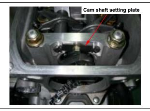
Install cam chain on to sprocket and align the timing mark on the sprocket with that of cylinder head.
