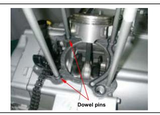
Coat some engine oil on inside of cylinder, piston, and piston rings.
