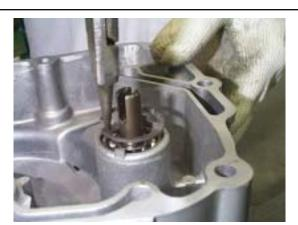
Check for any wear and damage of the mechanical seal and inside seal.
