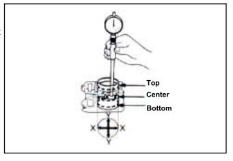
Check to see if cylinder is warped.
