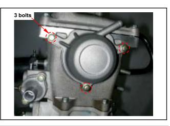
Remove left crankcase cover, and turn the drive face. Align the timing mark on the sprocket with that of cylinder head, piston is at TDC position.
