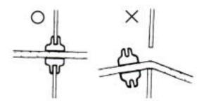
Never use wiring or harnesses if insulation has been broken. Wrap electrical tape around the damaged parts or replace them.
