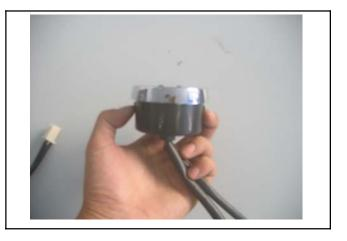
c. Install new meter and press down in to the meter casing.
