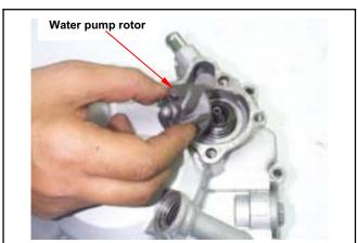
Install the dowel pin and right cover gasket. The rotation water pump impeller, causes the water pump drive shaft scoop channel, aligns the oil pump drive shaft flange, install the right crank case. (9 bolts)
