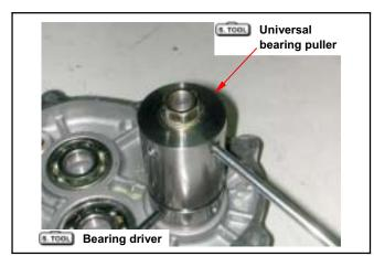
Install new oil seal and bearing driver into gear box covers inner side.
