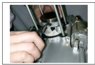
Remove cylinder gasket and dowel pin.
