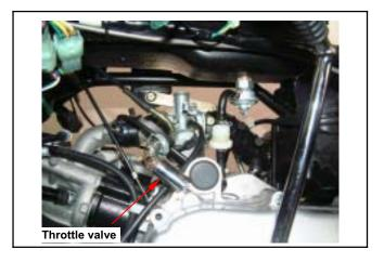
Disconnect the throttle cable from the throttle valve and remove the valve spring. Remove the fuel needle clamp and fuel needle.
