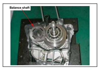
Remove crankshaft from right crankcase.
