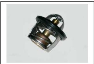
Place the thermostat into heated water to check its operation.
