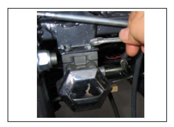
Turn off fuel petcock, then pull out the fuel intake line.
