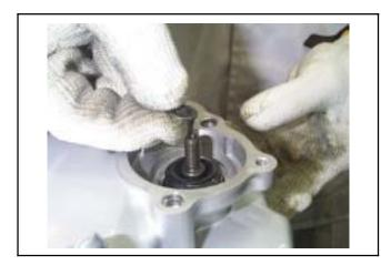
Install the impeller onto the water pump shaft and tighten.
