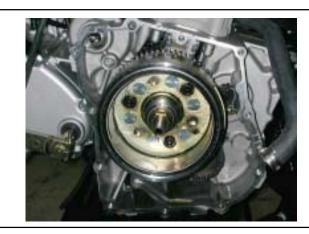
Install reduction gear shaft and reduction gear.
