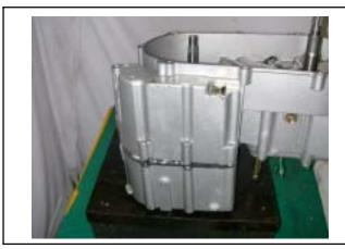
Tighten 11 bolts on the left crankcase. **Torque value: 0.8~1.2kgf-m**
