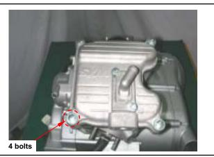
Install Air Injection system (AI) pipe. (4 bolts) Install inlet pipe onto cylinder Install and tighten spark plug
