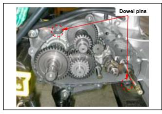
Install gear box cover and bolts, and tighten. Torque value: 1.0~1.4kgf-m
