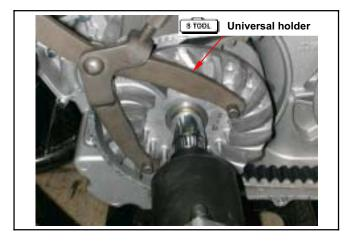
Remove movable drive face comp and drive face boss from crankshaft.
