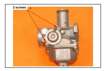
Remove air cut-off valve cover, spring and valve.
