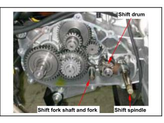
Remove final shaft, counter shaft, and reverse shaft.
