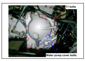
Connect water hoses to the right crankcase cover and water pump cover.
