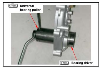
Turn the universal bearing puller to install drive shaft bearing.
