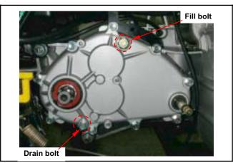
Remove gear box cover bolts (9 bolts) and then remove the cover.
