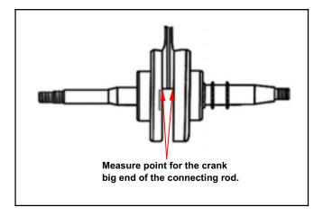
Measure the clearance of the large end in the vertical direction.
