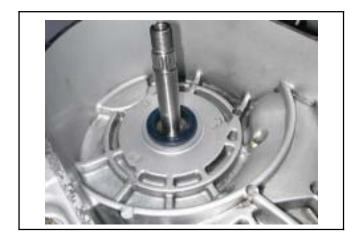
Apply by oil seal driver (27×42×7), oil seal will knock into location.
