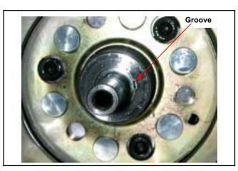
Hold the flywheel by drive face with universal holder, and tighten flywheel nut.
