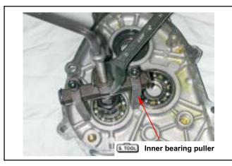
Remove cir clip of final shat out side bearing.
