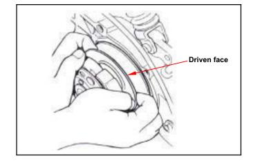
Install the driven pulley with belt onto drive shaft. Install the drive belts other end over the movable drive face.
