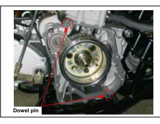
Remove water pump cover. Install right crankcase cover onto the crankcase. Note: Align the water pump shaft indent with the oil pump shaft.
