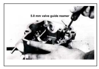
Measure and record each valve guide inner diameters.
