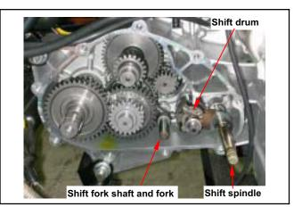
Install shift drum fixed catch ball, spring and bolt, onto gear box.
