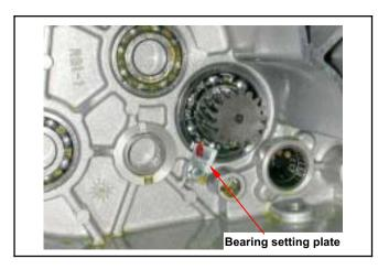
Remove the drive shaft. Special tool: **Shaft protector** Remove gasket and dowel pin.
