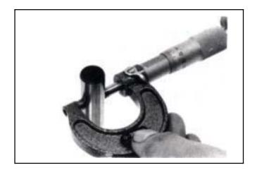
Measure the inner diameter of connecting rod small end.
