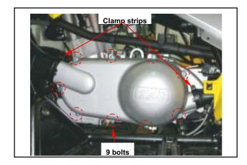
Check to see if the belt is cracked or worn out. Replace the belt if necessary or in accordance with the Periodic Maintenance Schedule.
