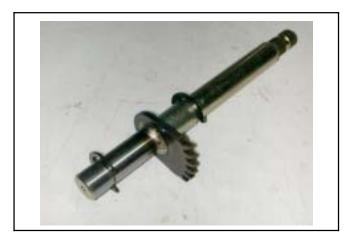
Check if the shift drum is worn or damaged.
