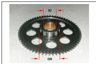
Check the starting reduction gear and shaft for wear or damage.
