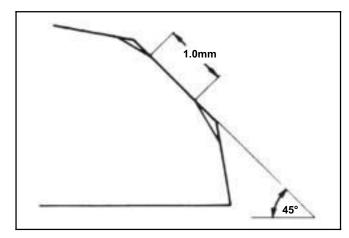
Coat the valve seat surface with red paint. Install the valve through the valve guide until the valve is contacting the valve seat. Slightly press down the valve but do not rotate it, so that a seal track will be created on contact surface.
