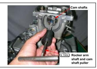
Remove the 2 cylinder head mounting bolts from cylinder head right side, and then remove 4 nuts and washers from cylinder head upper side. Remove the cylinder head.
