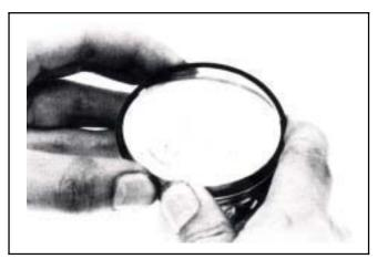
Place piston rings into cylinder below 20 mm of cylinder top, respectively. In order to keep the piston rings in horizontal level in cylinder, push the rings with piston.
