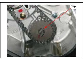
Install starting gear and generator. (Refer to chapter 9)
