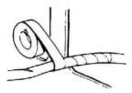
Secure the rubber boot firmly when applying it on wiring harness.
