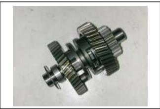
Check to see if the reverse shaft is worn or damaged.
