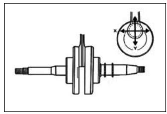
Place the crankshaft on a V-block, measure run-out of the crankshaft.
