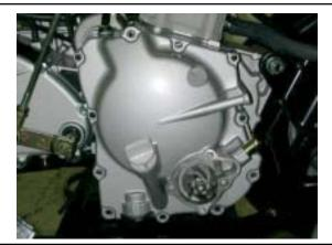
Install right crankcase cover (11 screws). Install the dowel pin, new gasket and water pump cover onto crankcase cover.
