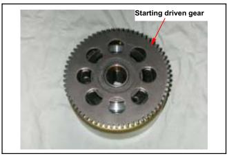
Remove 3 socket bolts, and then remove one way clutch.
