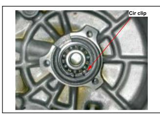
Remove the cir clip, and then remove bearing.
