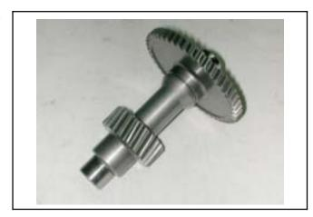
Check to see if the final shaft and gear are burnt, worn, or damaged.
