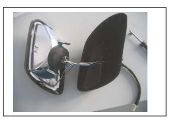
Remove wiring connectors.
