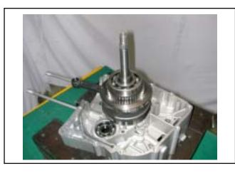
Align the position mark on the balance shaft drive gear with that of balance shaft driven gear, and then install balance shaft onto right crankcase.
