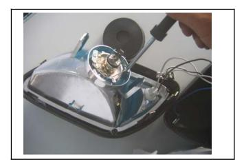
Install dust boot and wiring connectors.
