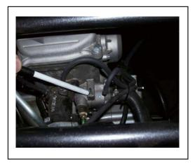
3. Continue to fill the radiator until the coolant level reaches the top of the radiator neck where the cap goes. After several minutes of idling the coolant level will drop. Refill the radiator to the same level and monitor for several more minutes for air bubbles. If the coolant level drops again, refill. Once the coolant level is stable and you no longer see air bubbles, screw the radiator cap back on and fill the reservoir to the appropriate level.
