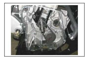
Remove cir clip and take out oil pump driving chain and sprocket.
