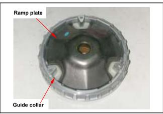
With 4~5g grease wipe drives in the movable drive face axis hole. Install drive face boss.
