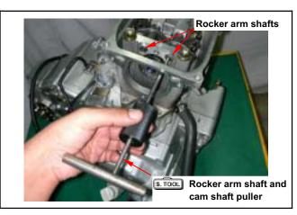
Remove cam shafts.
