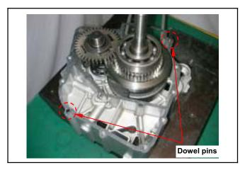
Install the left crankcase onto the right crankcase.
