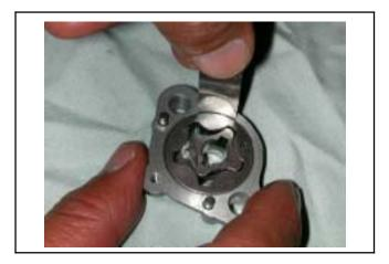
Check clearance between inner and outer rotors.
