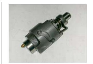
Check if the shift fork and shaft is worn or damaged. Measure the outer diameter of shift fork shaft, and replace it if it exceeds service limit.
