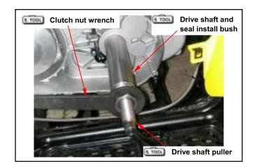
Apply with grease onto new drive shaft oil seal lip, and then install the oil seal.
