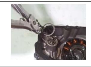
Install the seal washer into the impeller.
