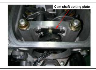
Remove rocker arm shafts and rocker arms. Special Service Tool:
