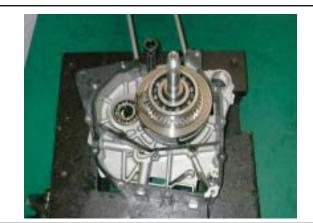
Remove gasket and dowel pins. Scrape gasket residues off the crankcase contact surface.
