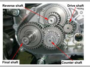
Remove drive shaft bearing setting plate (1 bolt).
