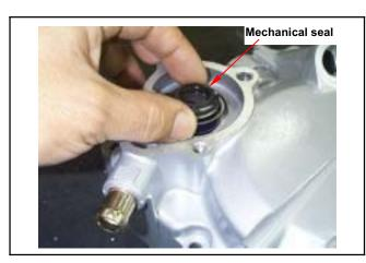
Install the mechanical seal onto the right crankcase.
