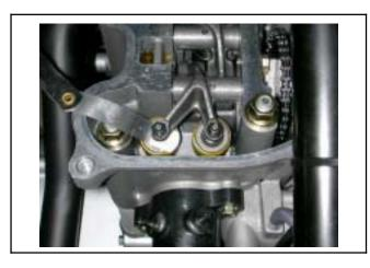
Remove the cylinder head side cover. Remove left crankcase cover, and turn the drive face, and align the timing mark on the cam
