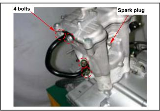
Remove the side cover mounting blots of cylinder head, and then take out the side cover.
