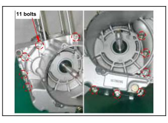
Tighten 2 bolts on the right crankcase. **Torque value: 0.8~1.2kgf-m**
