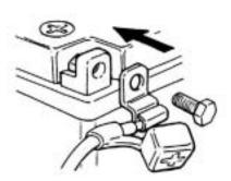
Make sure that the battery post caps are located properly after the battery posts have been serviced.
