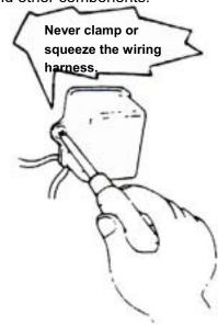
Do not let the wiring harness get twisted during installation.
