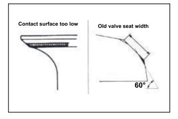
After the valve seat is ground, coat valve seat surface with emery and then slightly press the ground surface.
