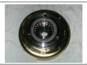
Install starting clutch driven gear onto one way clutch.
