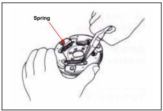
Install snap ring and mounting plate onto setting pin.
