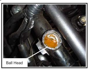
d. Fill steering gear box with grease after cleaning the dust. Replace the ball joint if it is loose or not smooth.
