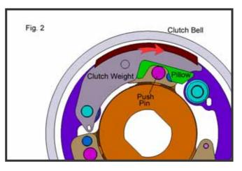
contacting with the bell, and the push pin is unactuated.] ,The friction resistance is produced between the clutch wear pad and the inner surface of clutch bell during the stage of slippery clutch-in.
