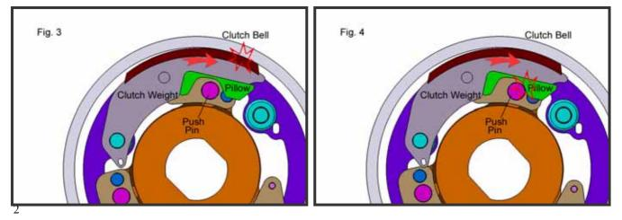
When the friction resistance is higher than the predetermined distortion strength of pillow spring, the pillow spring will be deformed or extended, and the Push Pin will thrust into the Pillow [Fig.4, the push pin is actuated and pressed against the pillow] to compress the clutch weight to grab the clutch bell/outer very tightly.
