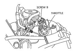
Carburetor Idle Adjustment Detail
