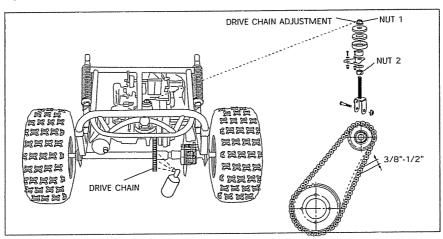
A new chain will have initial stretch and therefore will require adjustment. The first chain adjustment should be made after the first 2 hours of use. If the chain has more than ½" of slack or "flex" than it will require adjustment. To adjust:
