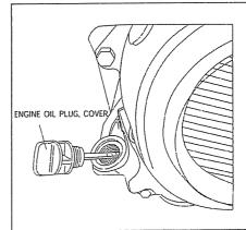
plug cap. Be sure to check the oil level before each use of the kart. Add oil when necessary to keep the oil level between the bottom of the dipstick and the "O" mark. NOTE: Oil level should be checked by dipping the oil level stick into the crankcase WITHOUT screwing the cap in.
