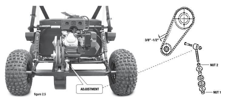
A new chain will stretch within the first few hours of use and therefore will require adjustment. The first chain adjustment should be made after the first 2 hours of use. If the chain has more than ½" of slack or "flex" then it will require adjustment. To adjust:
